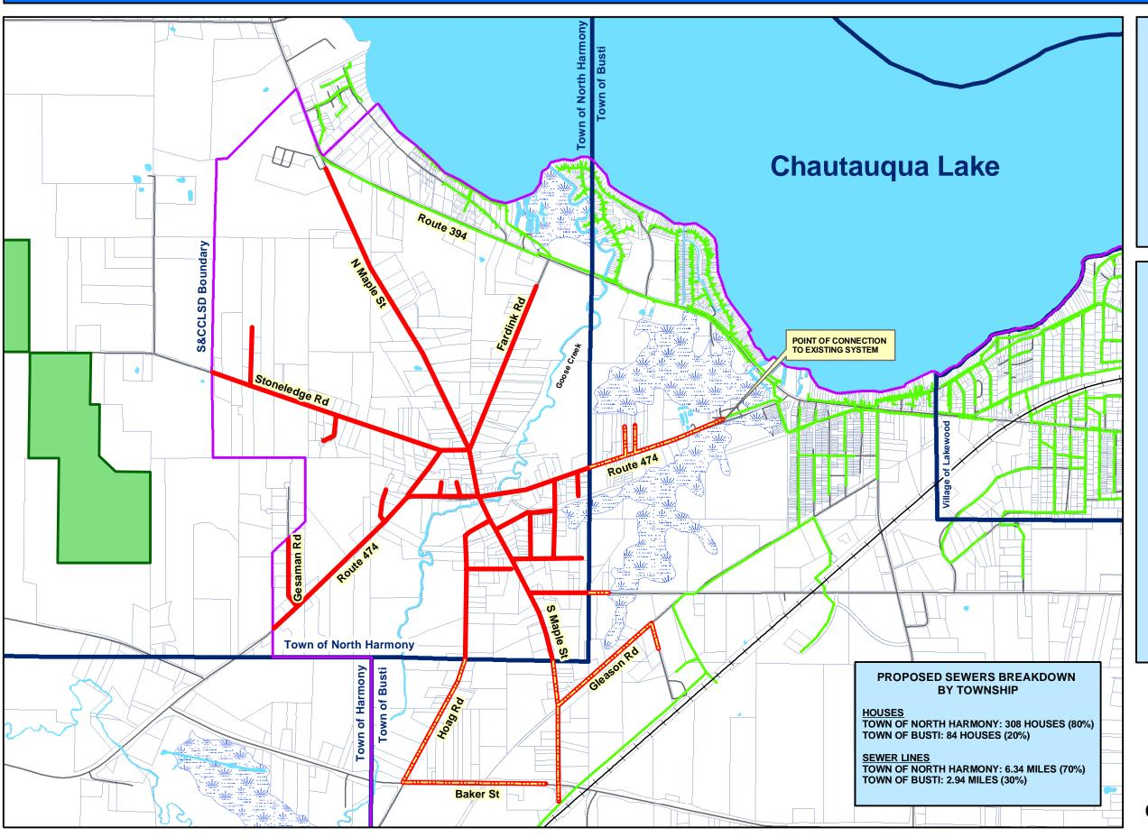
THIS PROJECT IS WITHIN THE PRESENT SCCLSD SERVICE AREA. THE RED LINES REPRESENT WHERE SEWER LINES WOULD NEED TO BE INSTALLED TO SERVE THE 392 HOMES AND BUSINESSES LOCATED IN ASHVILLE. THE TOTAL LENGTH OF PIPING IS ABOUT 9.28 MILES. THIS PROJECT IS A PROPOSED CONCEPT BASED UPON PRIOR SEWAGE FACILITIES STUDIES. THIS MAY BE SUBMITTED FOR CONSIDERATION TO FUND UNDER THE FEDERAL ECONOMIC STIMULUS PROGRAM.
