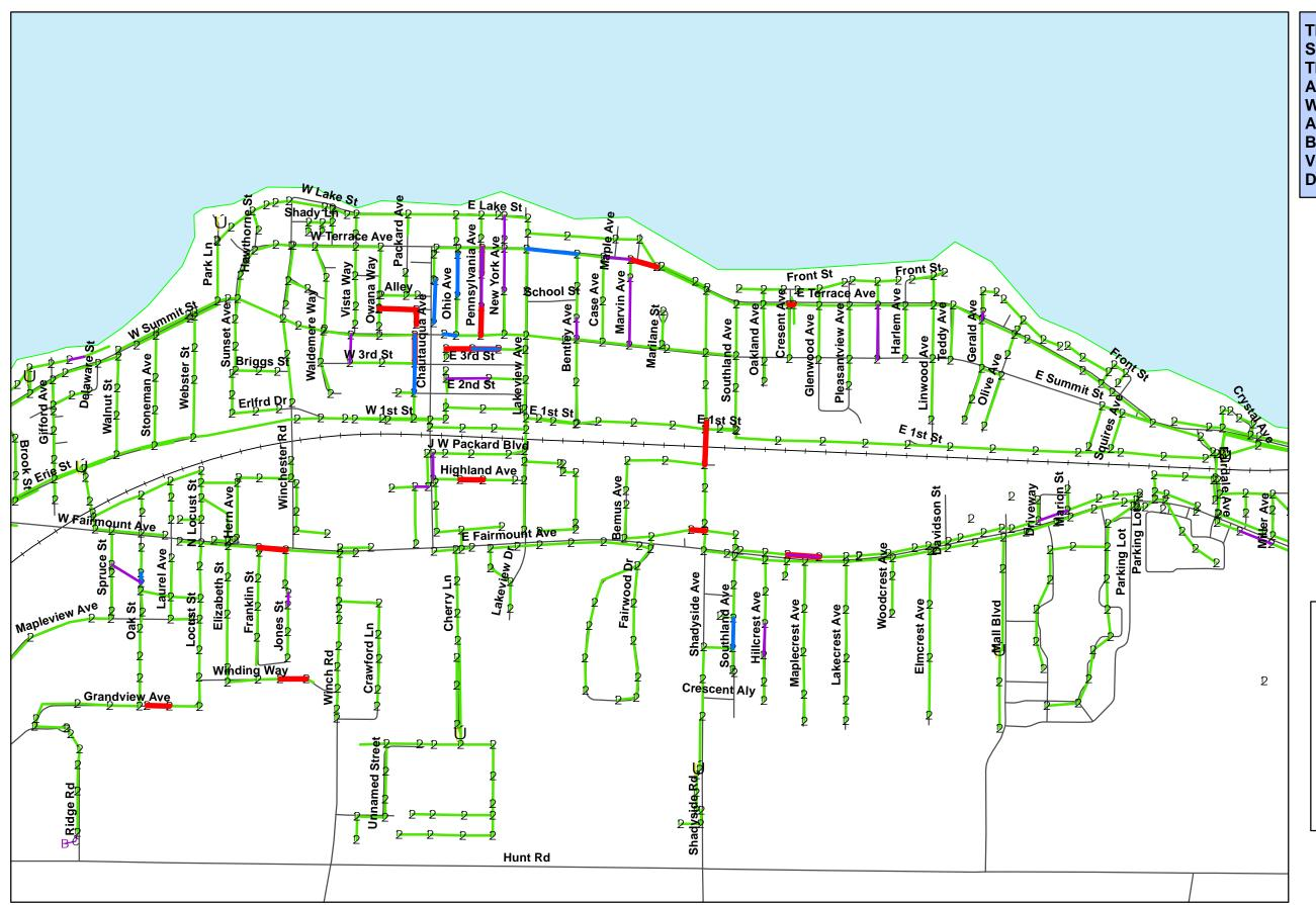
This Map Shows The Locations Of Sewer Main Breaks In Need Of Repair Throughout Lakewood. The Breaks Are Graded On A Scale Of 1 To 5 With Grade 5 Being The Most Severe And Grade 1 Being The Least Severe. Breaks Were Determined By CCTV Visual Inspection And Grades Were Defined By NAAPI And CATT.
